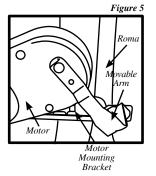
Follow all operating and assembly instructions for the Roma as before, except now instead of turning the handle, simply turn the **Motor** ON by selecting either slow speed (Setting I) or high speed (Setting II).
